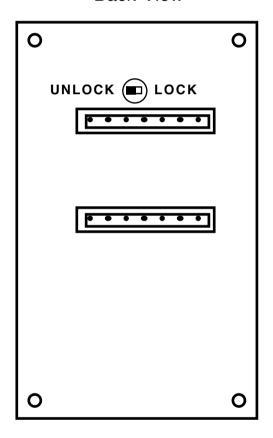
The Tamper Proof switch **LOCKS OR UNLOCKS** the front ENTER button. When the switch is to the LEFT, as shown, data can be entered or changed using the ENTER button on the front setup panel. When the switch is to the right, the ENTER switch is disabled and no data can be changed using the front setup panel.
