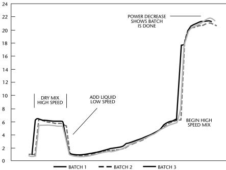
Note that for the three batches run, the curves don't vary much. A deviation from this profile should raise a red flag. Also, since power is linear with load changes it is easy to interpret and extrapolate the results at both the low and high end.
