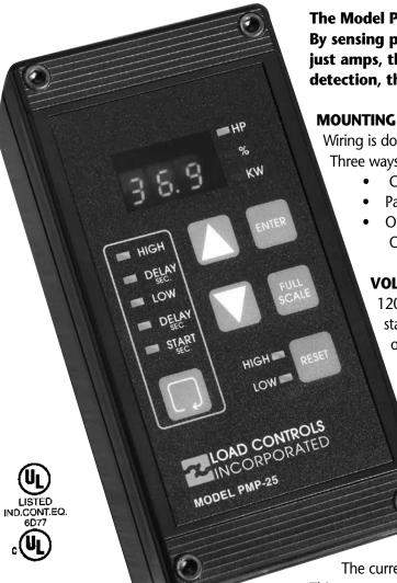
The Model PMP-25 monitors the true power going to a motor. By sensing power (volts x amps x power factor) rather than just amps, there is much greater sensitivity. For loss of load detection, this means a 10X improvement in performance.
