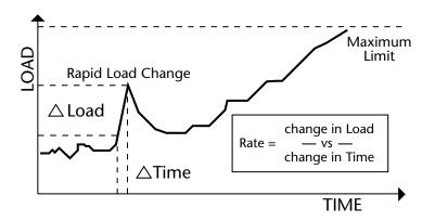
But, this is only half the equation. Jam-ups can occur even when the conveyor is lightly loaded. These rapid changes in load can also do damage. So, in addition to the maximum load limit, a "rate of load change" set point is needed to protect against problems when equipment is lightly loaded.
